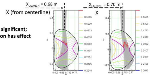
3: Top-launched beams will undergo greater refraction due to the non-normal incident angle, and may limit effective heating to density  $n_{e0} \leq 0.3 \times 10^{19}$  m<sup>-3</sup>.
