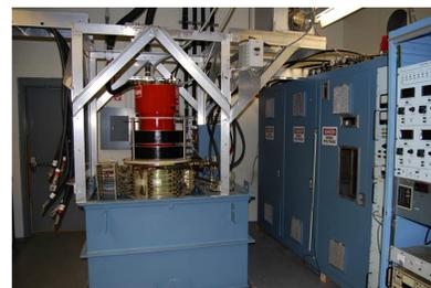
200kW, 28GHz Gyrotron (above) and designed beam hardware for side-launch configuration (right).
